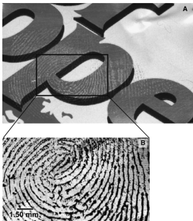
FIG. 2—Cut and flattened Dr. Pepper's soda can with fingerprint deposit. (A) Soda can imaged by a document scanner. (B) Infrared image of the outlined area obtained by plotting the band intensity at  $1016\text{ cm}^{-1}$ .
